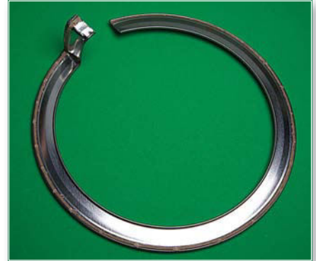
Fig. 5: The ring, split and bent to shape. The 'foot' bend is 6-10mm wide, and the other bend in the opposite direction, to form the 'knee' when assembled is 25mm from the foot bend.
