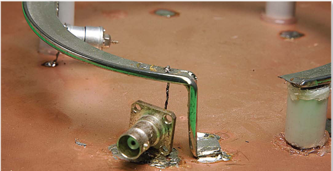
Fig. 6: The feed-point of the inner of the BNC socket is attached about 12mm from the knee bend of the antenna element. When I build another version, I'll mount the BNC socket from the underside of the p.c.b. material.
